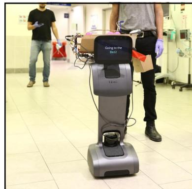
Rafael took a robot made by the TEMI company and placed multiple intelligent capabilities on it, enabling it to become a fully autonomous system that comes into close contact with COVID-19 patients in place of nurses. The robot,
